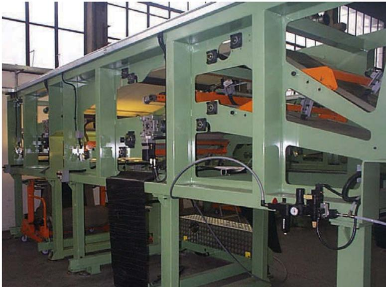
constant material tension during the various stages of application. Any spiral winding patterns can be programmed into the machine recipes.
