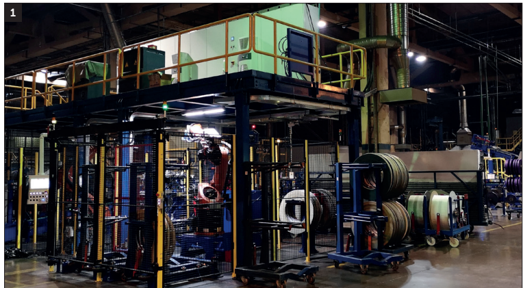
Figure 1 Intereuropean has developed the bead Apex Chipper & Flipper Assembly System for truck/bus tire plants
