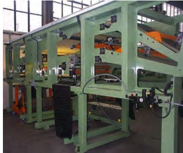
with Allen Bradley or Siemens PLC components. A touchscreen MMI is provided as standard, with graphic interface and dedicated screens for every machine function, recipe management, alarm handling and production statistics.
