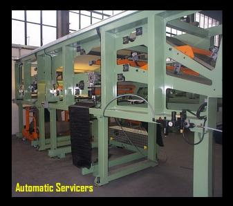
The Intereuropean Uni-Stage TBMs provide a fully automatic solution for building high performance tires with uni-stage technology.
