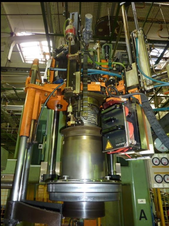
Upgrade of old Tire Testing Lines (Force Variation / Geometry / Balancing)
