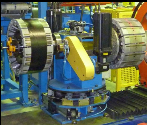
2nd Stage TBM Upgrade Twin Drums Turret
